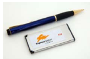
Figure 5: ExpressCard modules are smaller and lighter than previous PC Card and CardBus options.
