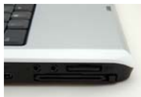
Figure 3: The ExpressCard slot comes in two sizes. The slot (left) is for ExpressCard/34 modules. A slightly wider slot, called the Universal slot, (right) supports both ExpressCard/34 and ExpressCard/54 modules.
